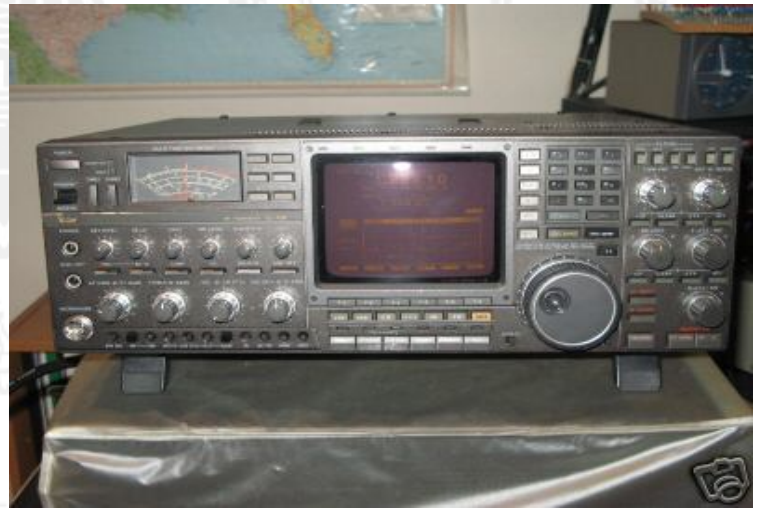
The Icom IC-781 as seen on E-Bay. This rig was way ahead of its time with that CRT display.
